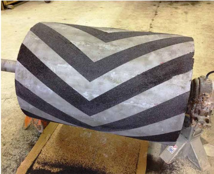
Belzona 1821 (Fluid Metal) is a grip system used to bond Belzona 9211 (Supergrip), Belzona 9221 (Surefoot White) or Belzona 9231 (Surefoot) to the surface of machinery and equipment.
